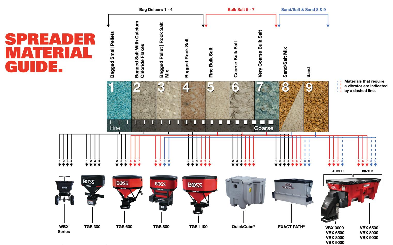
**NOTE:** Assumes dry, free-flowing material. Vibrators should not run continuously. The selection of proper deicing materials can be complex and varies by personal preference, experience and environmental concerns. All factors should be considered before making your selection.
